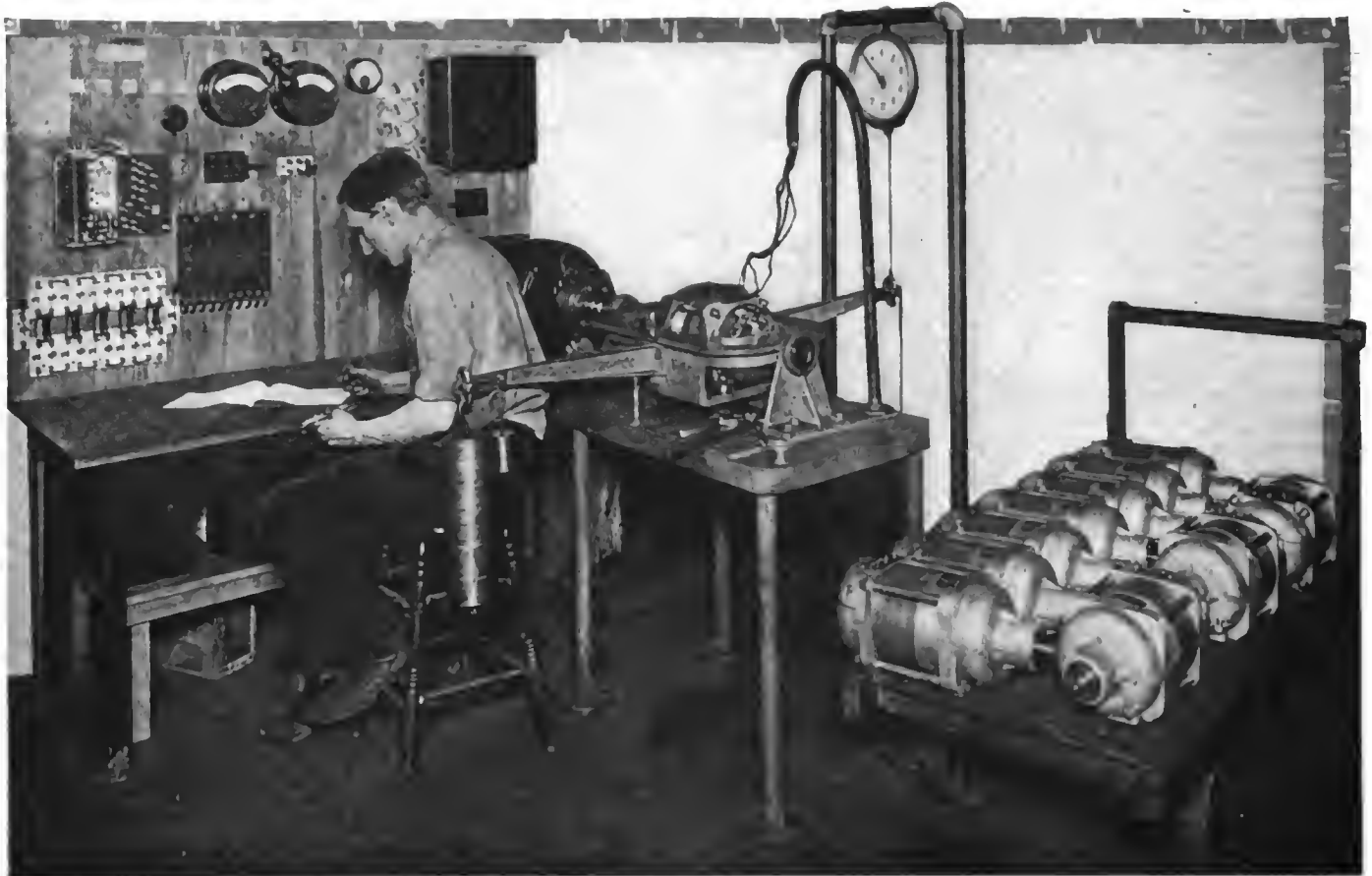
Testing apparatus used to determine the efficiency of the Apco starting and lighting system in the factory at Dayton, O.
